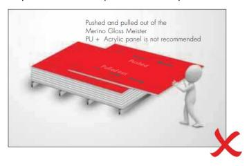
• When loading/unloading Gloss Meister panels, ensure the panels are lifted cleanly and don't scrape or slide over each other.
