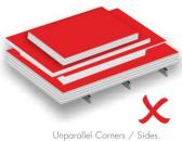
• Merino Gloss Meister panels should be absolutely parallel to each other in the rack and should not be stored in contact with walls or the ground.
