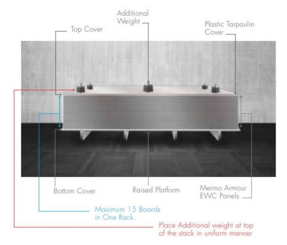
• While stacking Merino Gloss Meister High Gloss PU + Acrylic Panels, place a protective laminate over the top and under the bottom panel. Usually the stacking of Gloss Meister panels in supply of up to 15 boards is done with one sheet of 2mm or thicker laminate each at the bottom and similar laminate on the top. The top cover in all cases should be placed with some additional weight at appropriate places and in uniform manner.
